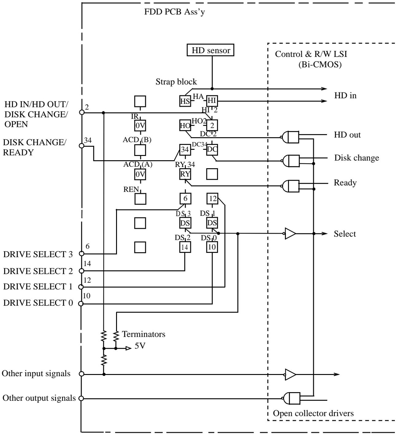
(Fig. 8.2-1) FDD signal interface circuit
